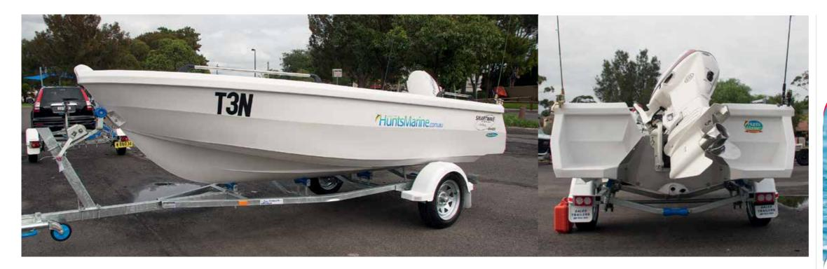
**Power:** The Smartwave SW4200 is rated for single, long-shaft motors of 30-50hp and certainly gave us quite nice speed results with an Evinrude 40hp ETEC.
